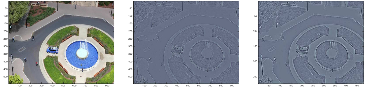
Figure 3: The first frame from the Neovision2 37 Tower sequence 011, which has been downsampled by a factor of two, where left is the resulting 960 \times 540 pixel RGB image, middle is the greyscale and pre-processed (see main text for details) version of the same image, and right is the image after additional factor of two downsampling (i.e. dimensions of 480 \times 270 pixels) followed by the same pre-processing.
